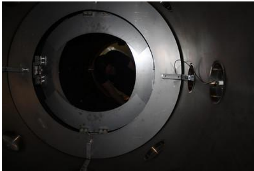
Limiters viewed from within plasma chamber
